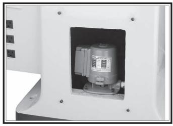
Figure 57. Location of coolant pump.
